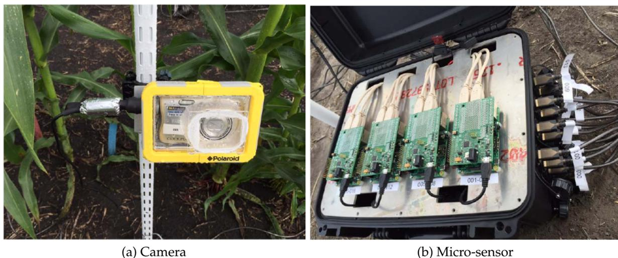
Figure 3.1: Photos of water-proof stationary camera and micro-controllers installed in the fields
